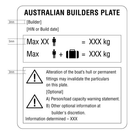
Figure A.8—Sample ABP template for boats 6 metres or more in length, not designed to be powered by an outboard engine using text and symbols
