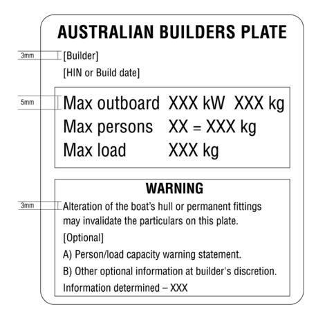
Figure A.5—Sample ABP template for boats 6 metres or more in length, designed to be powered by an outboard engine
