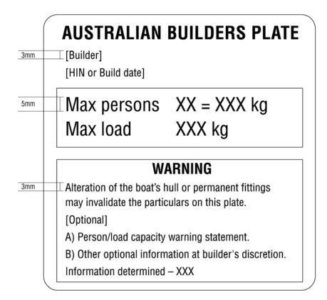
Figure A.6— Sample ABP template for boats 6 metres or more in length, not designed to be powered by an outboard engine
