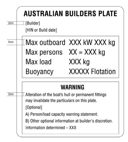
Figure A.1—Sample ABP template for boats less than 6 metres in length designed to be powered by an outboard engine
