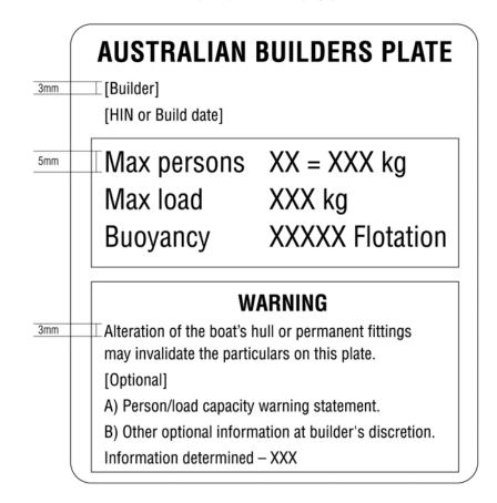
Figure A.2— Sample ABP template for boats less than 6 metres in length, not designed to be powered by an outboard engine
